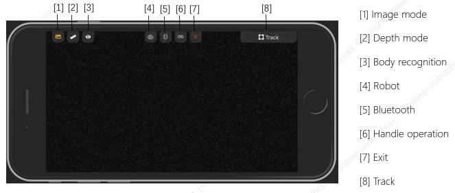
When the robot is in motion mode, click on the open tracking button to enter the character tracking interface, select the person to be tracked in the image, and the robot will follow automatically. Do not track missions in scenes with complex terrain or many obstacles.
