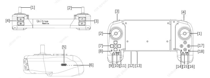
[1] Right Stick [2] Left Stick [3] L1/L2 Button [4] R1/R2 Button [5] Charging Interface Type C [6] Data transmission Signal Light [7] Left Button [8] Power Connection indicator [9] F1 (Left Stick Calibration Button) [10] SELECT Button [11] Charging Status Indicator [12] Battery Power Indicator [13] Power Button [14] Data Link Indicator [15] F3 (Right Stick Calibration Button) [16] START Button [17] Right Button [18] Bluetooth Signal Indicator
