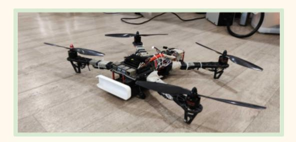
RaspberryPi based QuadRotor (Intel T265 based)
