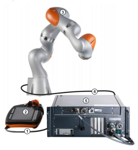
Fig. 3-1: Overview of robot system
