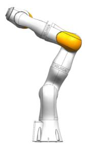
Fig. 7-1: Robot in transport position
